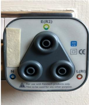
Mains socket-outlet access plug to facilitate safe connection of 4mm test leads.
