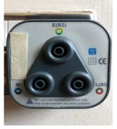
Mains socket-outlet access plug to facilitate safe connection of 4mm test leads. This can be used for the earth to EBB resistance test and the live to live voltage test (for two phases). Locally
